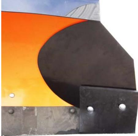
6. Verify the plow's cutting edge is on the ground. Hold the rubber cutting edge tightly against the ground, the Pro-Wing and plow's cutting edge. Mark location of the two holes in the bottom of the Pro-Wing on the rubber cutting edge from the rear and drill two 5/8 holes. Secure the rubber cutting edge to the Pro-Wing using 1/2" carriage bolt, 5/8" flat washer and nuts.
